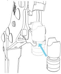
Apply LOKPREP 65G (02) onto the tube end of tube 1 (Cu suction line). Respect the curing time of the LOKPREP 65G (02).
