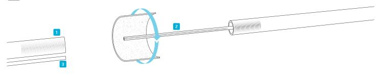
Apply LOKPREP 65G **(02)** onto the complete length of the insertion depths of the capillary tube and the Al suction line of **tube 2**.
