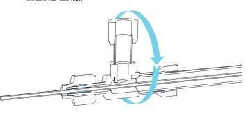
Position the jaws of the hand assembly tool (04) squarely onto the rings of the LOKRING NTR connector (03). In a controlled manner use the hand assembly tool (04) to press the rings onto the connector ensuring that the insertion depth of the tubes does not change throughout this process. Once both rings are flush to the centre stop of the connector the joint is complete, remove the hand assembly tool (04) from the LOKRING NTR connector (03).
