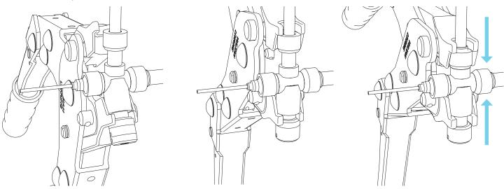
Connect tube 3 (capillary tube) according to the assembly instructions for LOKRING® tube connection assembly version 00 on www.vulkan.com.
