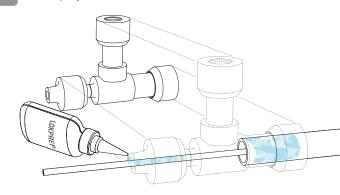
Push the LOKRING NTR connector (03) onto tube 2 and rotate the LOKRING NTR connector (03) through 360° to distribute the LOKPREP 65G (02) evenly. Respect the curing time of the LOKPREP 65G (02).
